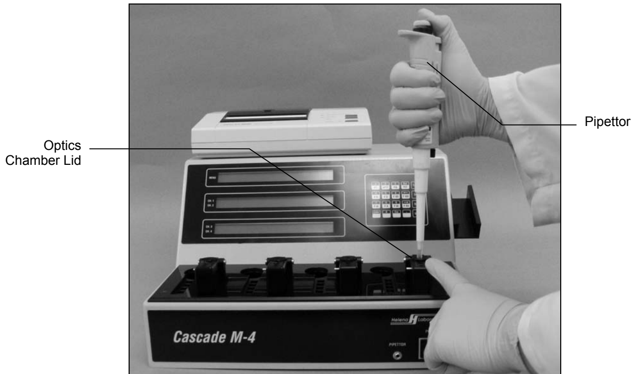
Figure 6-2. Simultaneously Press Optics Chamber Lid and Pipette Reagent
